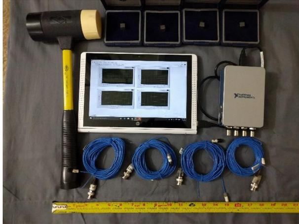
**Figure 10:** Equipment used for EDAR testing.
