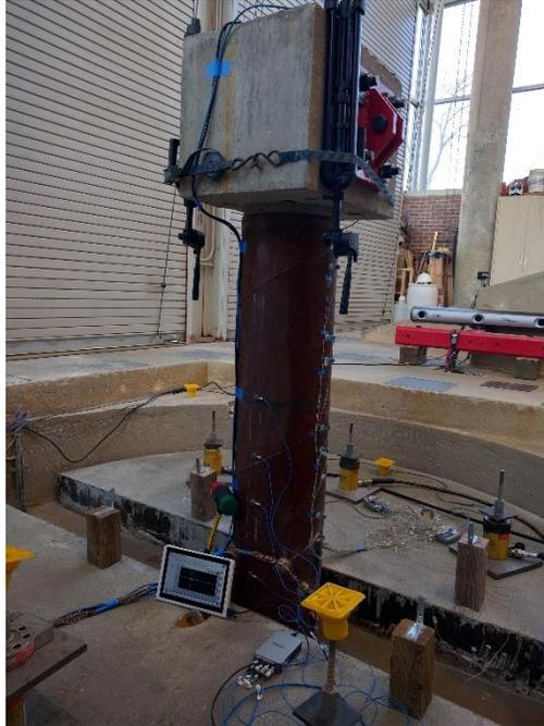
**Figure 9:** Concrete filled steel tube tested at NCSU.
